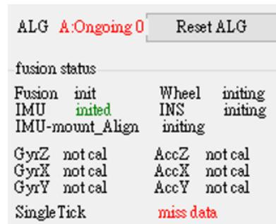
ALG is abbreviated for alignment. It transits from **Ongoing** to **Coarse** and then **Fine** during calibration process.
